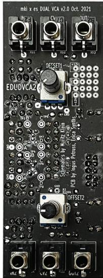
**Insert the potentiometers, but don't solder them yet!** Fit the front panel and make sure that the potentiometers' shafts are aligned with the holes in the panel – and that they're able to rotate freely. Now, go ahead and solder the potentiometers.
