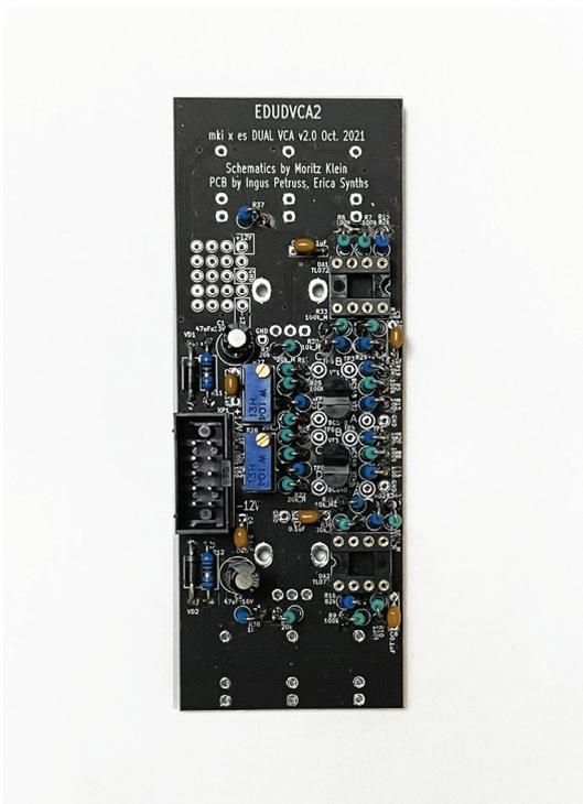
**Next, solder the precision trimmer and the power supply socket.** Make sure the orientation of the socket is as shown in the picture below – the arrow pointing to the first pin is aligned with a notch on the silk-screen. The key on the socket will be facing inwards to the PCB.
