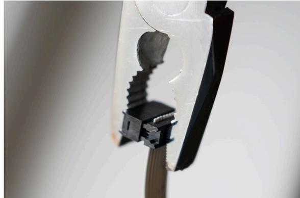
Figure 25: Fixation of the IDC connectors to the ribbon cable.
