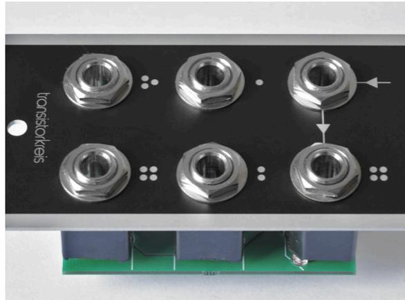
Figure 23: The fixed front panel jacks.
