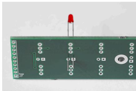
Figure 12: The rectangular solder pins for the LED cathode leads.
