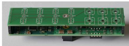
Figure 9: Forming a sandwich before soldering J7 and J8.
