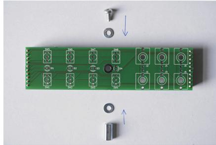
Figure 10: The spacer fixation.
