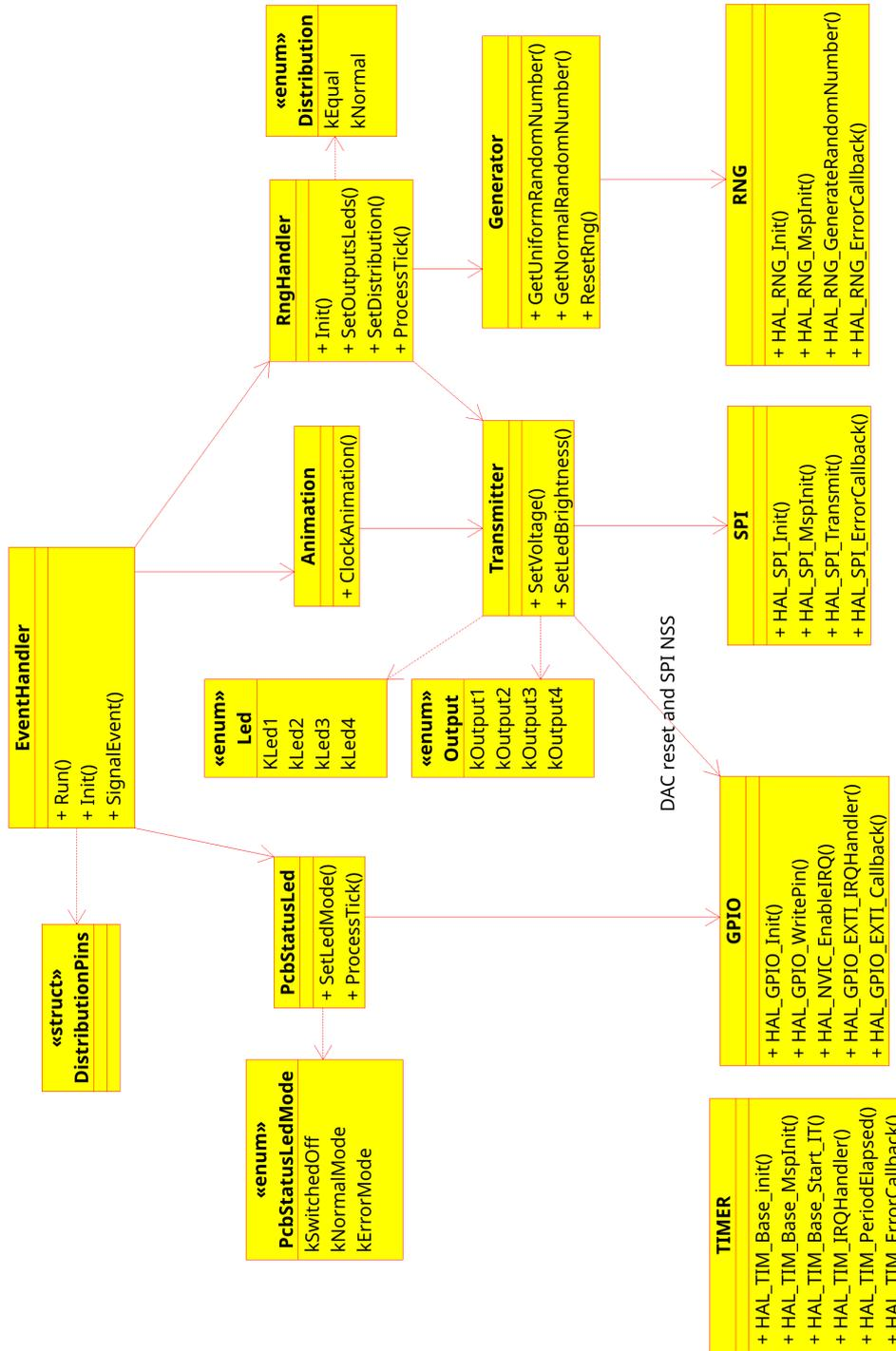
Figure 29: UML class diagram of the firmware
