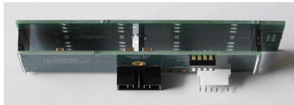
Figure 16: Forming a sandwich before soldering J1 and J2.
