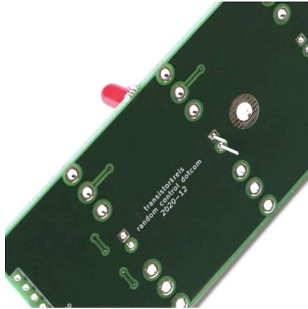
Figure 19: The rectangular solder pins for the LED cathode leads.
