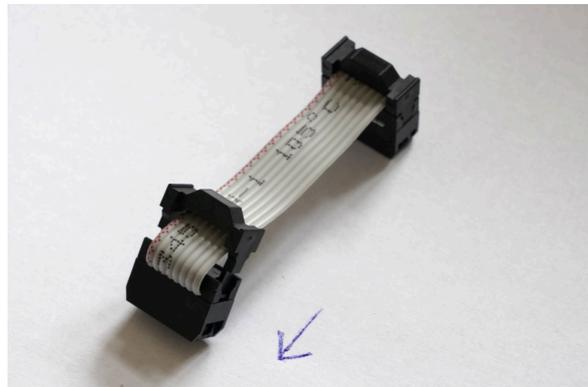
Figure 26: Additional fixation of the ribbon cable.
