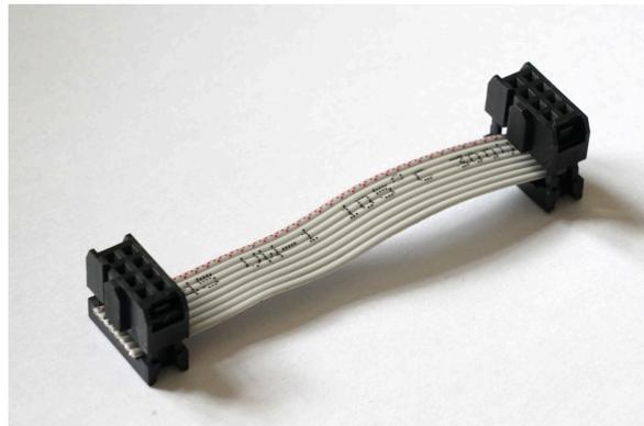
Figure 24: Orientation of the IDC connectors.
