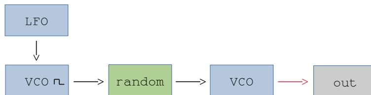
Figure 6: The random module as digital noise modulator.
