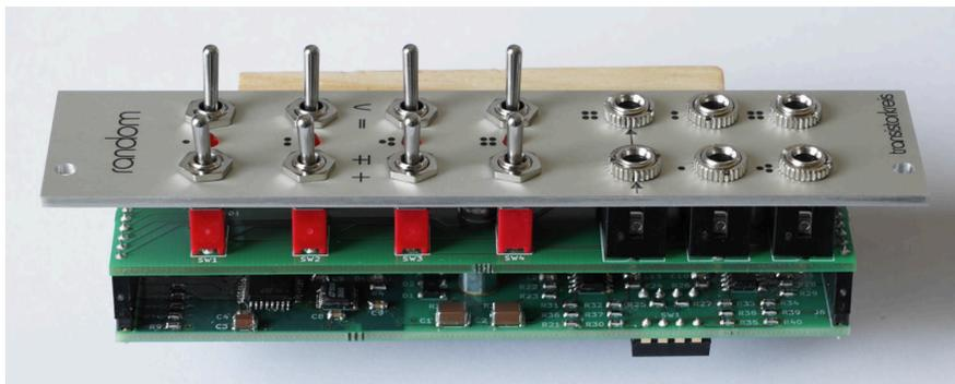
Figure 14: The ready-built Eurorack module.
