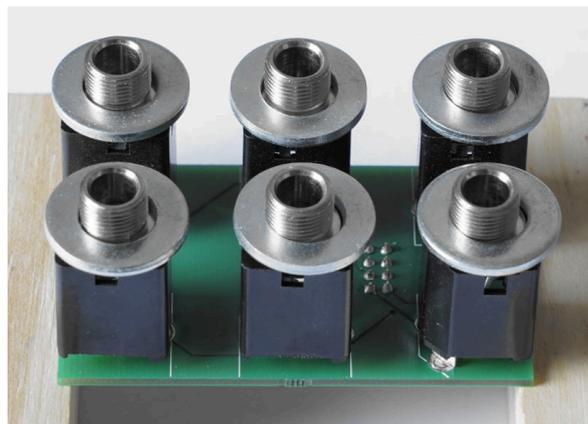
Figure 22: Washers placed onto the jacks.
