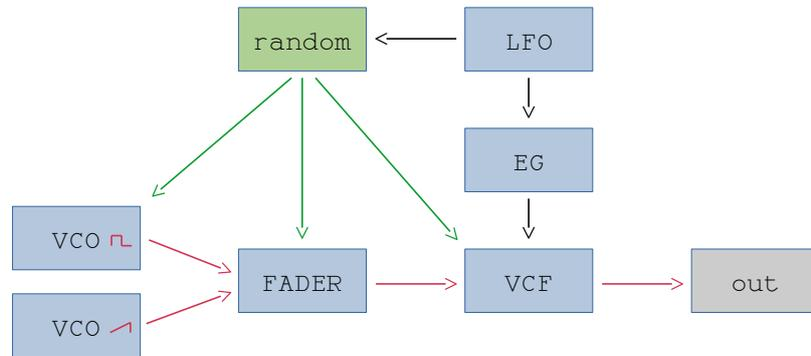
Figure 4: The random module as CV source.
