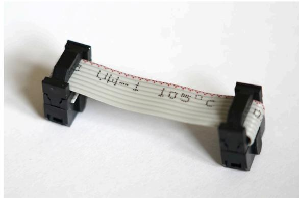
Figure 27: The ready-built ribbon cable.
