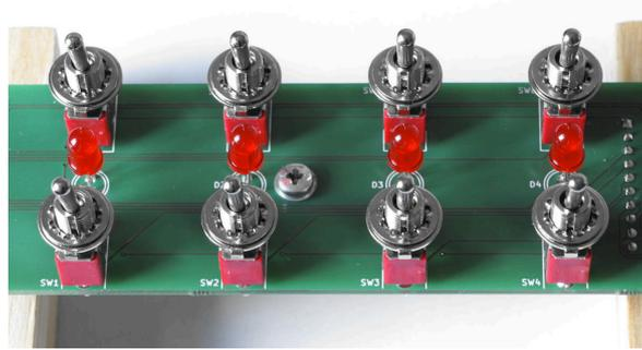
Figure 21: LEDs and switches placed onto the Control PCB.
