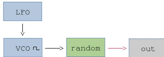
Figure 5: The random module as digital noise oscillator.
