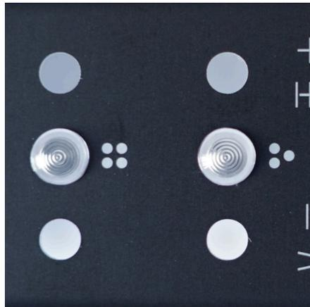
Figure 18: Front panel LED holders.
