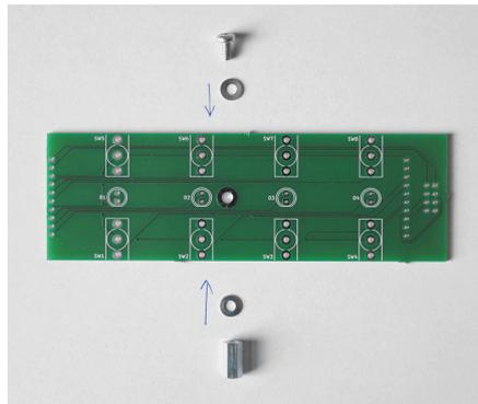
Figure 15: The spaceholder fixation.
