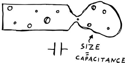
Then, should the pressure in the pipe drop, the balloon releases the water it stored into the pipe. The maximum size of the balloon is determined by the capacitor's capacitance, which we measure in farad (F). There are quite a few different types of capacitors: electrolytic, foil, ceramic, tantalum etc. They all have their unique properties and ideal usage scenarios – but the most important distinction is if they are polarized or not.
