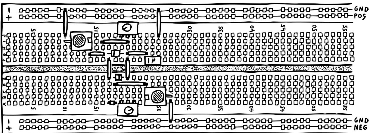
If you connect your LFO and VCF like before, you should be able to sculpt the filter movement much more freely by adjusting attack and release independently. So what we've built here is an ultra-simple passive attack-release envelope generator. Why passive? **Because it does not include any form of amplification.** It's getting all of its
