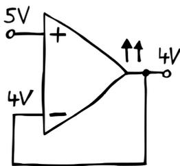
But as it's pushing up that output voltage, the **voltage at the inverting input will be raised simultaneously.** So the difference between the two inputs is shrinking down. Initially, this doesn't matter much because the gain is so large. As the voltage at the inverting input gets closer to 5 V though, the difference will shrink so much that in relation, the gain suddenly isn't so large anymore.
