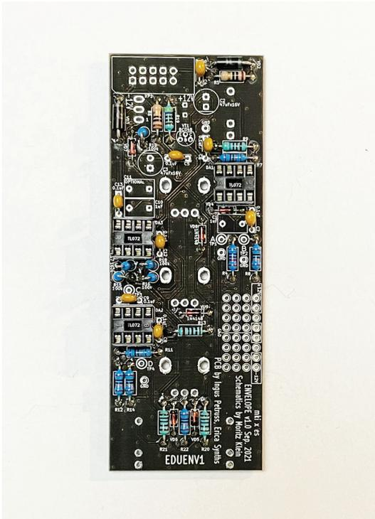
**Next, insert & solder the electrolytic capacitors.** Electrolytic capacitors are bipolar, and you need to mind their orientation. The positive lead of each electrolytic capacitor is longer, and there is a minus stripe on the side of the capacitor's body to indicate the negative lead. On our PCBs, the positive pad for the capacitor has a square shape, and the negative lead should go into the pad next to the notch on the silkscreen.
