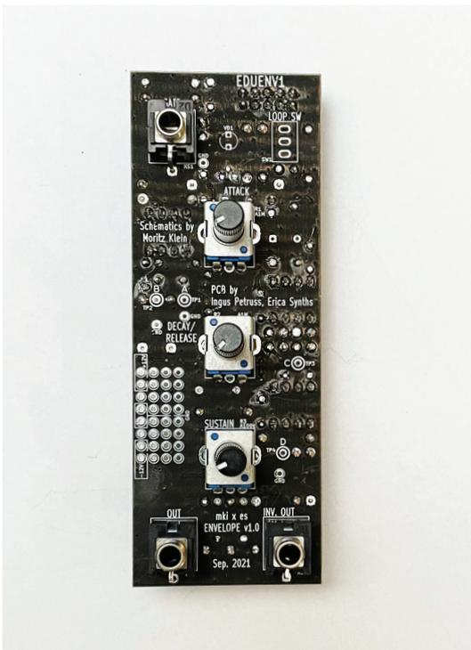
**Insert the potentiometers, but don't solder them yet!** Fit the front panel and make sure that the potentiometer shafts are aligned with the holes in the panel – and that they're able to rotate freely. Now, go ahead and solder the potentiometers.
