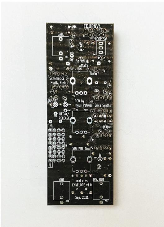
Now, turn the PCB around and inspect your solder joints. **Make sure all components are soldered properly and there are no cold solder joints or accidental shorts.** Clean the PCB to remove extra flux, if necessary.
