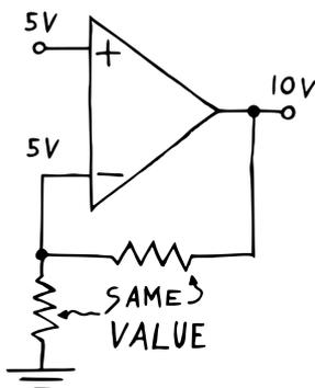
How about amplifying a signal though? To do that, we'll have to turn our buffer into a proper non-inverting amplifier. We can do that by replacing the straight connection between inverting input and output with a voltage divider, forcing the op amp to work harder. Here's how that works. Say we feed our non-inverting input a voltage of 5 V. Now, **the output needs to push out 10 V in order to get the voltage at the inverting input up to 5 V.** We call this setup a non-inverting
