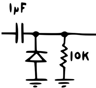
First a positive one, when the input transitions from low to high – and then a negative one when it drops from high to low. Now, since we're not interested in the negative spike, and it could cause our comparator to glitch out under certain circumstances, I've decided to eliminate it using another diode. Whenever the voltage at the comparator's input (i.e. after the 1 µF capacitor) tries to go negative, the diode will open and thereby neutralize it.<sup>12</sup>
