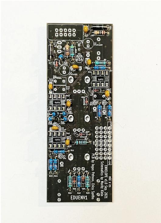
**Next, insert & solder the electrolytic capacitors.** Electrolytic capacitors are bipolar, and you need to mind their orientation. The positive lead of each electrolytic capacitor is longer, and there is a minus stripe on the side of the capacitor's body to indicate the negative lead. On our PCBs, the positive pad for the capacitor has a square shape, and the negative lead should go into the pad next to the notch on the silkscreen.
