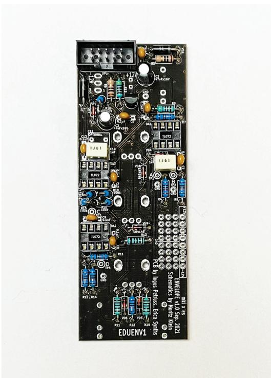
**Next up: inserting & soldering the transistor.** Make sure you align the transistor with the marked outline on the silkscreen – **orientation is critically important here.** Also, insert film capacitors and solder them.
