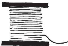
**Solder wire with flux.** I find 0,7mm solder wire works best for DIY projects.
