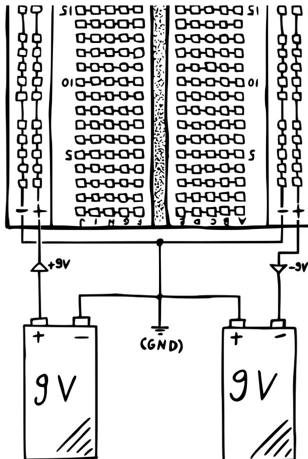
By connecting the batteries like this, the positive terminal of the left battery becomes your +9 V, while the negative terminal of the right is now your -9 V, and the other two combine to become your new ground.<sup>19</sup> **Please make sure you disconnect the batteries from your breadboard when you make changes to the circuit!** Otherwise you run the risk of damaging components.
