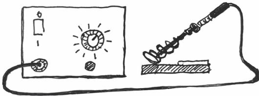
**A decent soldering station.** Top-of-the-line soldering stations (brands like Weller) will cost 200€ and above, but cheaper alternatives around 50€ are often good enough. Make sure your soldering station of choice comes with multiple differently-sized soldering iron tips. The most useful ones for DIY electronics are flat, 2mm wide tips.
