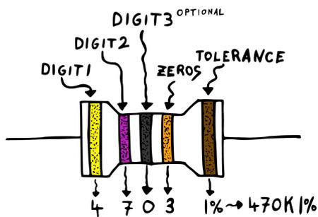
For the resistors in this kit, a yellow body tells you that the actual resistance value might be  $\pm 5\%$  off. A dark blue body indicates  $\pm 1\%$  tolerance. Some kits will also contain light blue  $\pm 0.1\%$  resistors to avoid the need for manual resistor matching.
