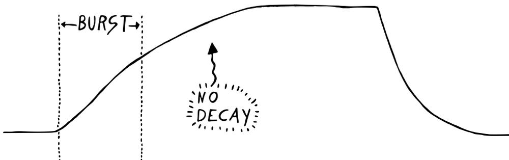
In effect, we basically skip the decay phase, as we are never dropping down to the sustain level. Now granted, a proper ADSR envelope shouldn't have these two problems. But for how simple our circuit is, and how few components it uses, I think we can book this as a worthwhile tradeoff. So let's set this up on the breadboard!
