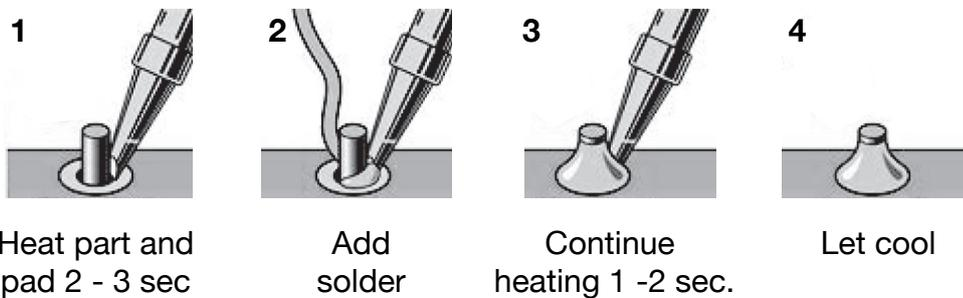
After you have completed soldering, inspect the solder joint:
