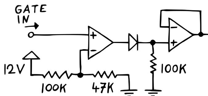
Here's what that does. Whenever the comparator is pushing out 12 V, the diode conducts and we also get about 12 V at the buffer's input. But once the voltage turns negative, the diode will block. Normally, the buffer's input would now be undefined (or „floating“). But since we have a 100k resistor to ground there, that input gets pulled down to 0 V instead.
