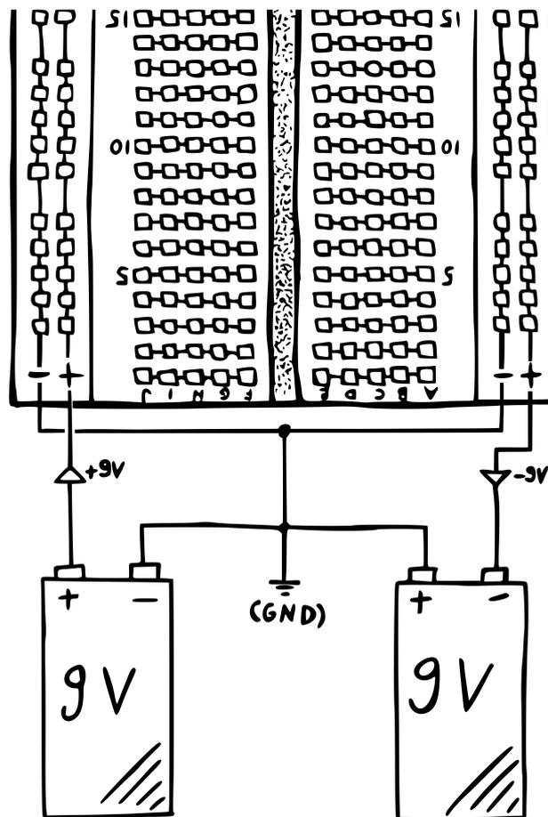
By connecting the batteries like this, the row on the left side labeled + becomes your positive rail, the row on the right side labeled + becomes your negative rail, and both rows labeled – become your ground rails.<sup>2</sup> **Please make sure you disconnect the batteries from your breadboard when you make changes to the circuit!** Otherwise you run the risk of damaging components.
