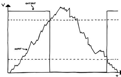
This works because a Schmitt trigger inverter has two thresholds against which it compares the voltage we apply to its input. The three resistors up top (or rather the relation between them) set those thresholds. In our case, the bottom threshold is set at 0 V, while the top threshold is placed at around 8 V. So when the input drops to 0 V, the op amp's output will jump to 12 V. Then once the input rises above the 8 V line, the output will drop down to -12 V.
