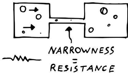
**Resistors have two distinctive properties: linearity and symmetry.** Linearity, in this context, means that for a doubling in voltage, the current flowing will double as well. Symmetry means that the direction of flow doesn't matter – resistors work the same either way.
