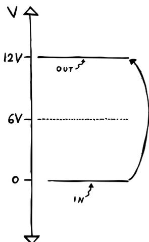
Turns out it's doable quite easily with another op amp, which we'll set up as an inverting buffer.<sup>15</sup> But instead of connecting the non-inverting input to ground – as you would normally do –, we give it a constant 6 V from a simple 50 % voltage divider.
