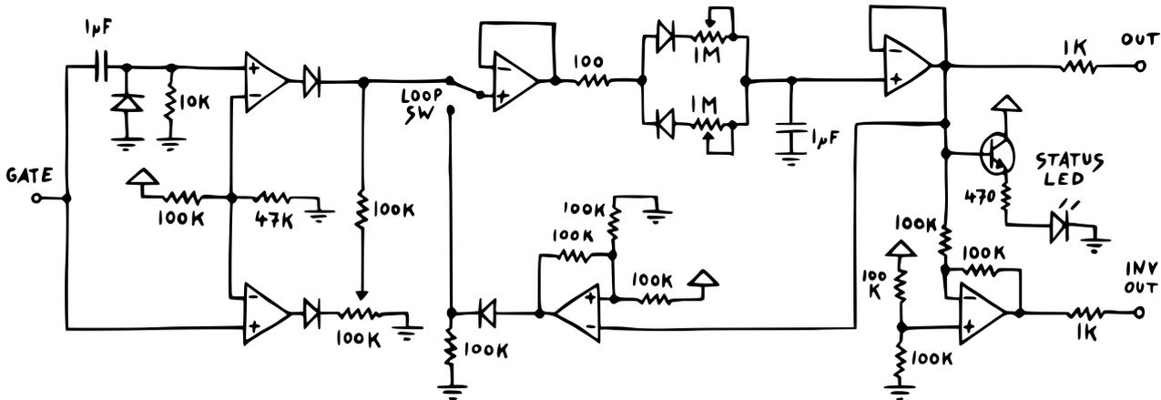
By circumventing the input comparators, the relation between our Schmitt trigger inverter’s state and the envelope’s output voltage becomes a lot simpler. Because now, there’s no envelope setting that can prevent its output from peaking at a value below 8 V. The inverter will simply keep pushing out a high level voltage until we cross that threshold.
