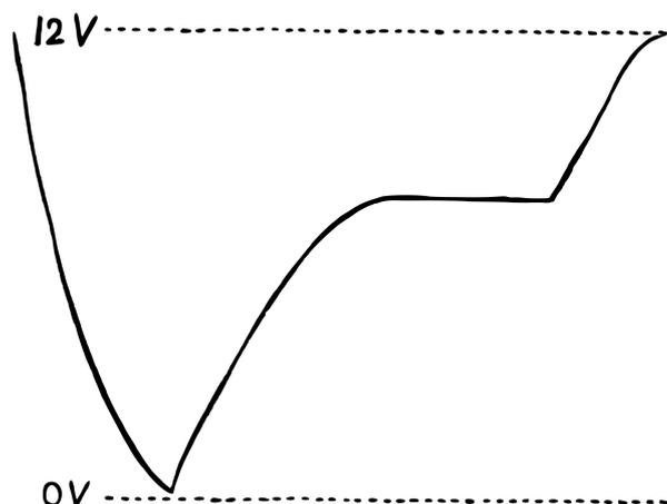
It's the same core principle, but the baseline is now our high level voltage. Meaning that the curve is no longer dipping into the negatives, but rather „peaking“ at ground level. This way, it'll do the exact opposite of what we've seen before when controlling a VCF with it. The filter will be wide open by default, and then close down as the envelope is cycling through its phases. Cool! But how do we actually implement this?
