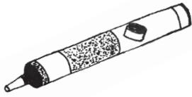
**A solder suction pump.** No matter how refined your soldering skills are, you will make mistakes. So when you'll inevitably need to de-solder components, you will also need to remove any remaining solder from the solder pads in order to insert new components.
