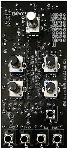
**Insert the potentiometers.** Don't mix up their values and **don't solder them yet!** Fit the front panel and make sure that the potentiometers' shafts are aligned with the holes on the panel – and that they rotate freely. Now, go ahead and solder the potentiometers.
