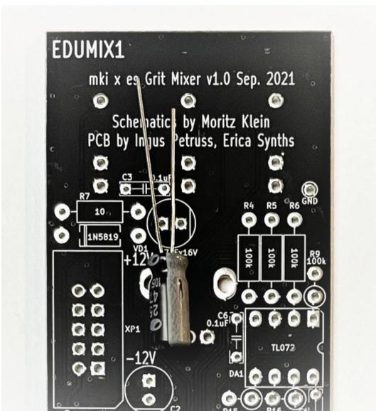
**Next, insert & solder the electrolytic capacitors.** Electrolytic capacitors are bipolar, and you need to mind their orientation. The positive lead of each electrolytic capacitor is longer, and there's a minus stripe on the side of the capacitor's body to indicate the negative lead. On our PCBs, the positive pad for a capacitor has a square shape, and the negative lead should go into the pad next to the notch on the silkscreen.
