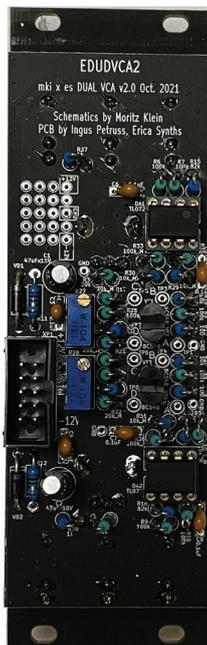
Now, **insert the ICs into their respective DIP sockets.** Mind the orientation of the ICs – match the notch on each IC with the one on its socket.
