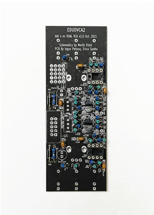
**Next up: inserting & soldering the transistors.** Make sure you place the transistors in their designated spots. Also, they need to be properly aligned with the marked outline on the silkscreen – orientation is critically important here.
