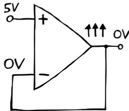
Before the op amp starts processing the voltages at its inputs, the output will be switched off. This means that **output and inverting input sit at 0 V at first.** So then, the op amp will subtract 0 from 5 and multiply the result by its gain. Finally, it will try and increase its output voltage to match the calculation's outcome.
