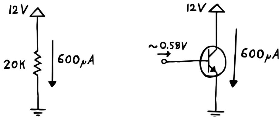
One is just a resistor between a voltage source and ground. The other is a transistor, with its collector connected to an identical voltage source, its base connected to another much weaker voltage source, and its emitter connected to ground. Now if we tune the base voltage carefully, we can get the exact same amount of current flowing through our
