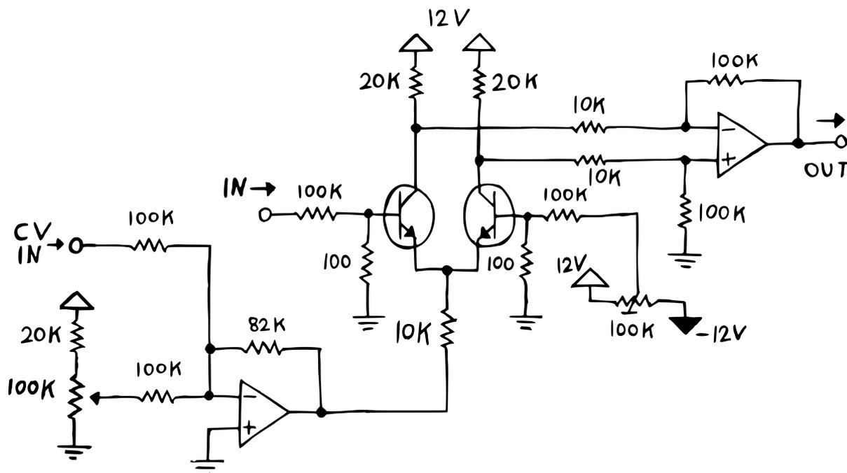
To fix this, we can simply use a bit of our subtractor op amp's gain. Because right now, we are really only using it to subtract our two signals – not to amplify the result. How do we change that? **By making the output work harder to equalize the two input voltages.** And in order to make it work harder, we have to change the relations between the resistors around the op amp.<sup>25</sup>
