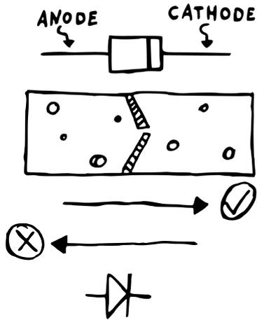
Diodes are basically like one way valves. Current can only pass through in one direction – from anode to cathode. That direction is indicated by the arrow in the diode symbol, and by a black stripe on the diode’s casing. So any current trying to move in the opposite direction is blocked from flowing.
