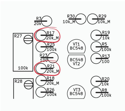
But as this is a pre-assembled kit and we didn’t want to just drop a big pile of resistors on your head, we pack it with **±0.1% tolerance resistors** where needed. Which means that there’s no real need for matching – they’re going to be close enough straight out of the box. You can identify these **±0.1% tolerance resistors by their light blue bodies** – use them wherever you see an M on the part placement diagram. If you’re unsure about a resistor’s value, use your multimeter to double-check.
