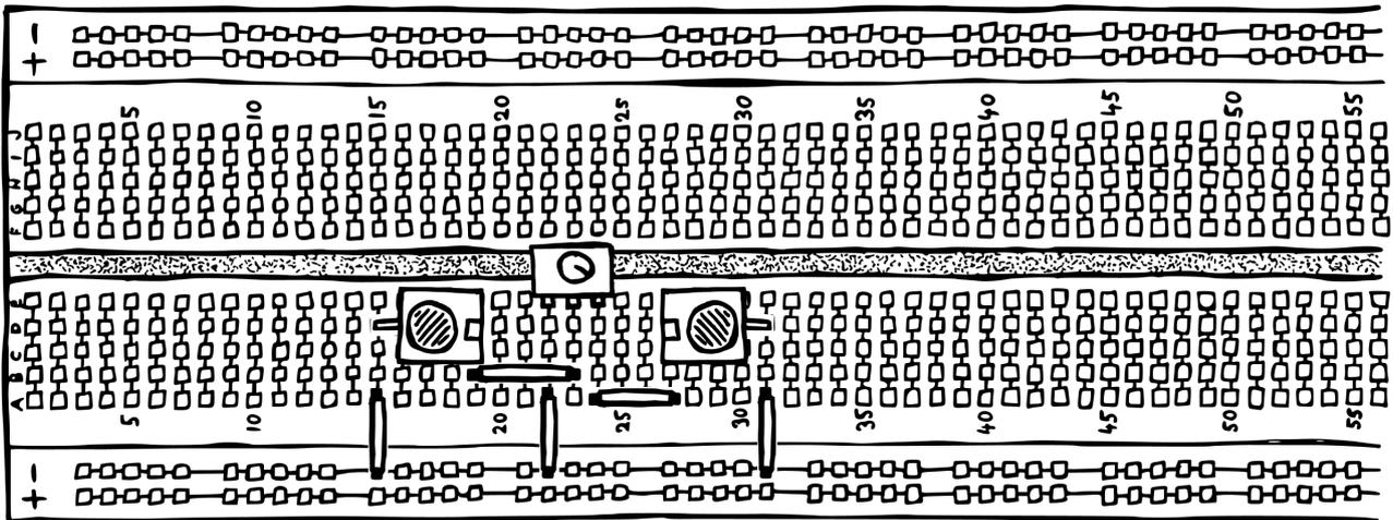
By turning the potentiometer, you should now be able to change the signal's volume.<sup>8</sup> With this, we know why voltage dividers are a good fit for manual volume control. **But the question is: how can we modify them to give us voltage-based volume control?** Well, if you've watched some of my earliest videos, you might already be thinking in a certain direction here.
