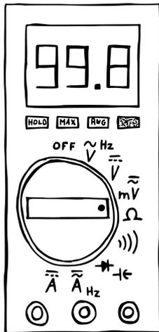
Multimeters come in different shapes and sizes, but the most common type is probably the hand-held, battery powered variant. These can measure a bunch of different things: voltage, current, resistance, continuity. Some have additional capabilities, allowing you to check capacitance, oscillation frequency or the forward voltage drop of a diode.
