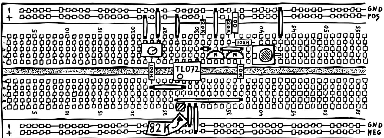
If you connect your oscilloscope to both collectors (on separate channels – or one after the other) and play with the potentiometer, you should be able to verify our assumptions.<sup>21</sup> Both signals are moving downwards as their volume increases significantly. Now if you zoom in a bit, you should see that they indeed are inverted copies of each other. Okay – but you might say: so what? How is having two signals with their DC offsets tied to the gain better than one?
