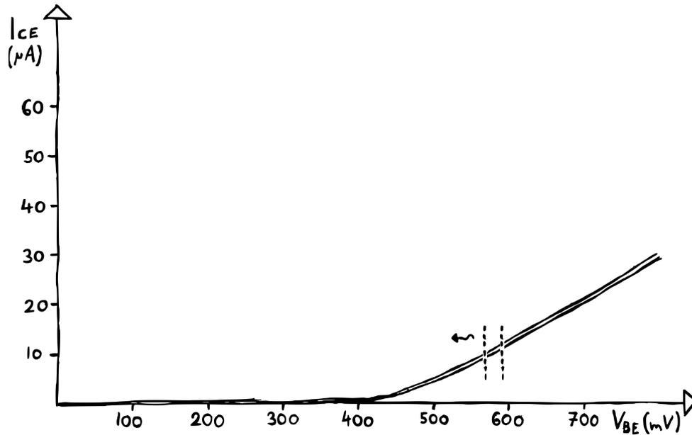
Since this will have a direct effect on our collector current swing, we should also see a reduction in gain. But while we could go through the trouble of adding our scaled-down input signal to a variable DC bias before applying the sum to the transistor's base, there is a simpler, more elegant solution.
