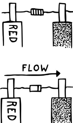
In some cases, it doesn't matter which probe you connect to which component leg or point in your circuit. This is true for testing resistors, non-polarized capacitors (foil/film, ceramic, teflon, glass etc.), continuity<sup>34</sup> or AC voltage.
