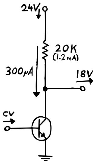
Which is precisely why the initial idea of a transistor-based voltage controlled voltage divider does not work. Since the current going through our transistor is fixed (if the base voltage does not change and the collector voltage stays positive), the total current flowing will be fixed as well. **So in- or decreasing the collector voltage will only change the potential, not the actual flow amount.**
