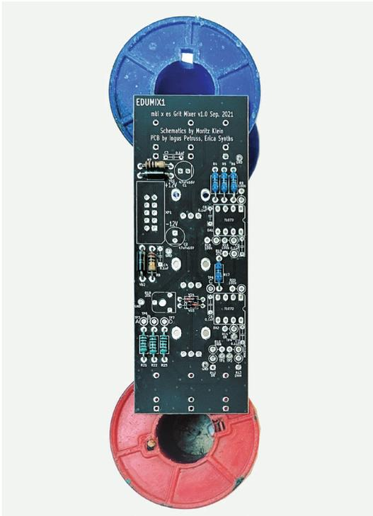
Place the dual VCA PCB in a PCB holder for soldering or simply on top of some spacers (I use two empty solder wire coils here).
