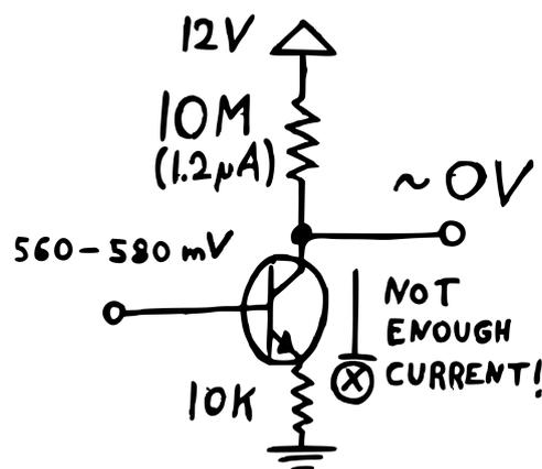
Because at some point the potential amount of current will drop below the set collector current, starving our transistor of power and distorting – or even killing – the oscillation at the output.
