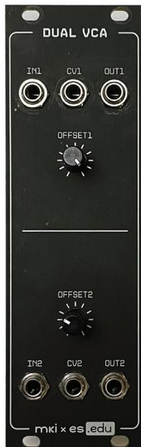
**Install the front panel** and fix it in place with the 6 hex nuts on the jack sockets. We are almost done!
