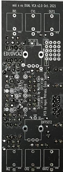
Now, turn the PCB around and inspect your solder joints. **Make sure all components are soldered properly and there are no cold solder joints or accidental shorts.** Clean the PCB to remove extra flux, if necessary.
