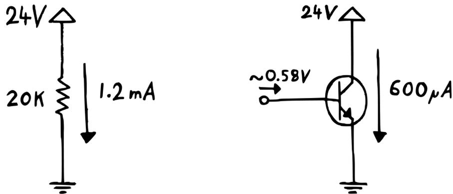
We'll still see the same 600  $\mu\text{A}$  flowing through this circuit. Why is that? **Because the only thing determining the amount of current that can flow between collector and emitter is the amount of current flowing into the base.** And the latter only depends on the voltage at the base – not the voltage at the collector. Now while this would already disqualify the transistor, let's also check for the second property: symmetry. What happens when the collector voltage goes negative?
