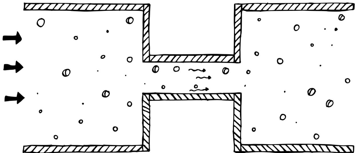
In that metaphor, resistance would be the width of a pipe. The wider it is, the more water can travel through it at once, and the easier it is to push a set amount from one end to the other. Current would then describe the flow, while voltage would describe the pressure pushing the water through the pipe. You can probably see how all three properties are interlinked: **more voltage increases the current, while more resistance to that voltage in turn decreases the current.**
