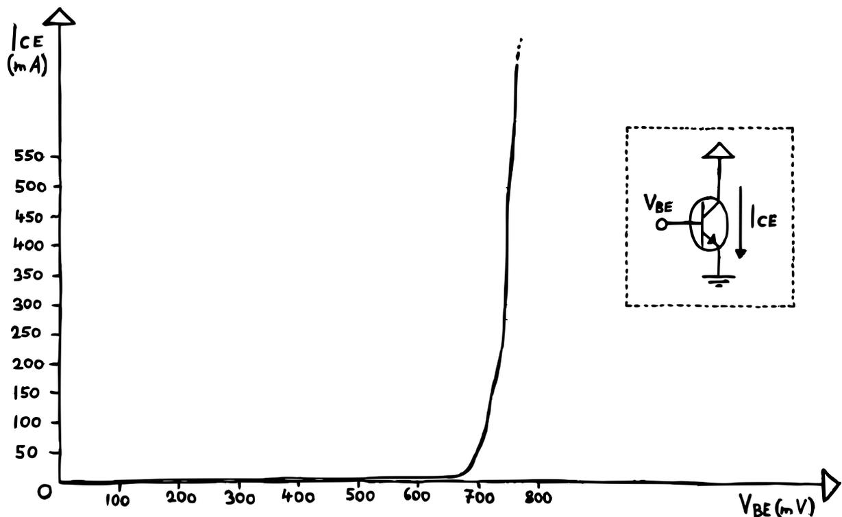
First, the relation between base voltage and collector current is exponential. Second, unlike a resistor, a BJT is not symmetrical – so we can't really reverse the direction of the
