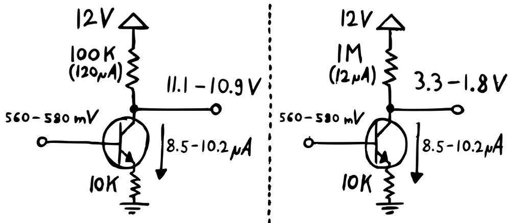
Because if we increase it, then we reduce the amount of current that could potentially flow through it. Now, since this does not affect the transistor's operation, the collector current swing will stay the same. Which means that essentially, it's swinging across a larger portion of the full potential, netting us a bigger voltage swing at the output. There is a hard limit here, though. **We can't just keep increasing the collector resistor's value in hopes of unlimited additional gain.**
