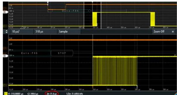
Next 2 pictures show MINICV response to MIDI note. The 2nd one shows re-trigger in action. In this case re-trigger was set to minimum duration, that is 0.1.ms. It is user configured up to 5ms. Orange trace is MIDI input decoded to hex numbers right below, green trace is Gate, and yellow trace is CV. As you can clearly see, CV is updated less than 200us after last bit of a note is received
